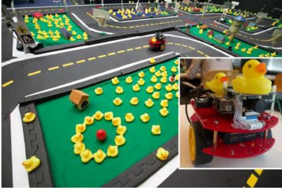
**Figure 1:** Duckietown is a scaled-down autonomous city where the inhabitants are duckies. The platform comprises autonomous vehicles (Duckiebots) and a well-specified environment in which the Duckiebots operate. This platform is used as the basis for the AI Driving Olympics competition which will take place at the NIPS 2018 conference.
